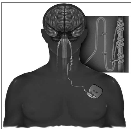
Fig. 1. Schematic representation of placement of the NeuroCybernetic Prosthesis manufactured by Cyberonics, Inc. for therapeutic left cervical vagus nerve stimulation.
